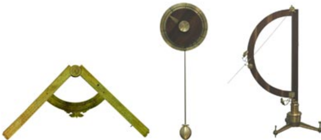
Figure 14: Other three Galilean objects displayed at the Laboratorio . From left to right: the geometric and military compass, the pulsilogium, and the apparatus for demonstrating the “theorem of the cords”.
