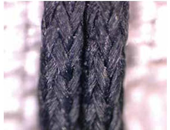
Black braided silk sutures, treated with wax and silicone, magnified 150-fold. Nicole Ong, Biomaterial Matters (2017).
